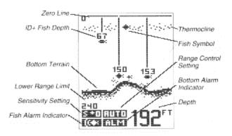
There are three basic screen layouts for the Wide W. Figure A shows the default screen layout which does not include temperature and speed readings. If you have purchased the temperature and speed accessory and it is installed, the screen layout will be slightly different as shown in Figure B.
